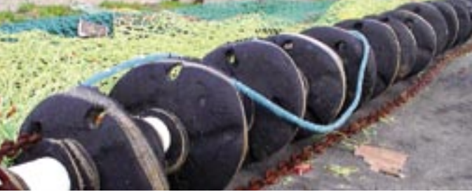
Bottom trawl roller-gear Source: © OCEANA / David Hall
