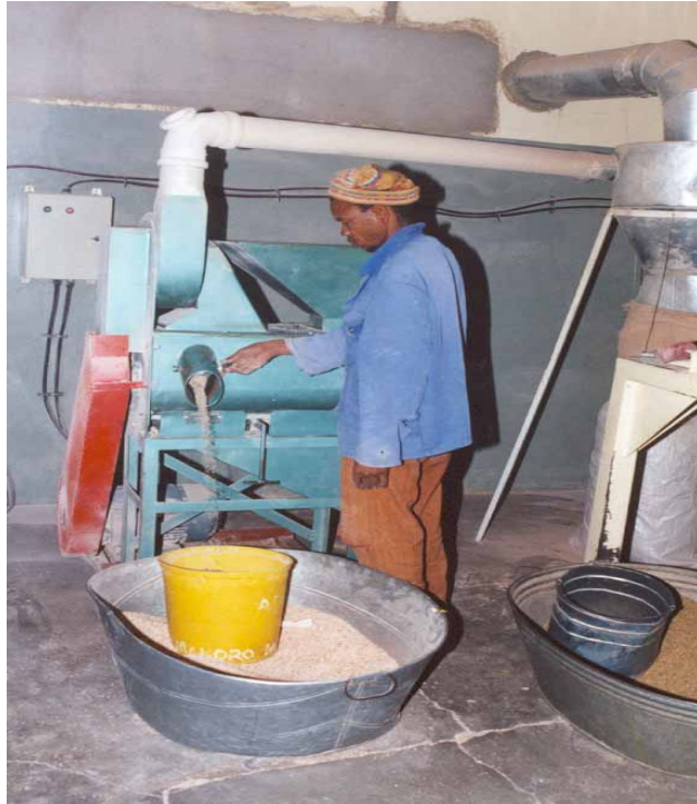
A sorghum dehuller developed by the Rural Industries Promotion Company
